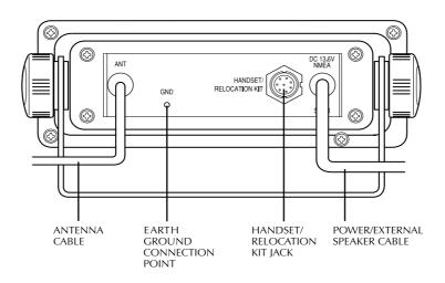
Figure 2-6 Typical Grounding Method
